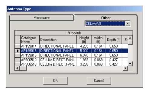
The data shown includes all parameters of these antennas necessary for the program to calculate wind loads and weight effects.
