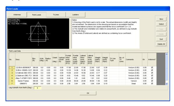
In this window the mast elevation is shown along with the plan cross-section at the point load elevation. To add a new point load select **New** and input line with zero values is shown. The user inputs the following data as defined below:
