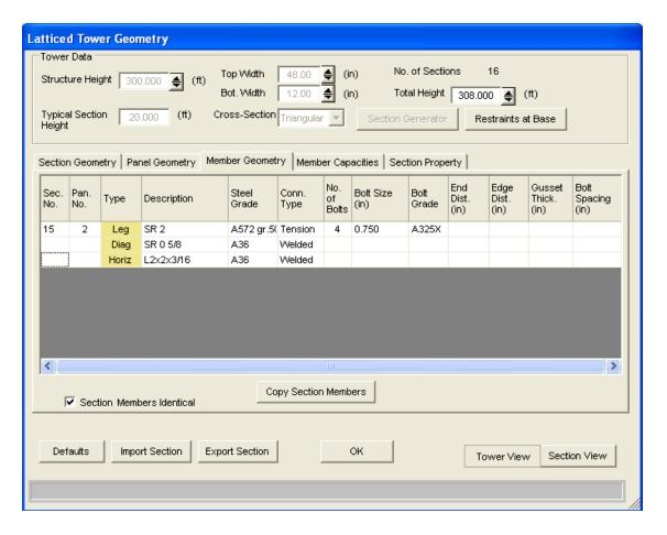
From the Member Geometry Screen, the user defines the member sizes, steel grades, connection type, number of bolts, bolt size, bolt grade, end distance, edge distance and gusset thickness. The following is a definition of the different fields:
