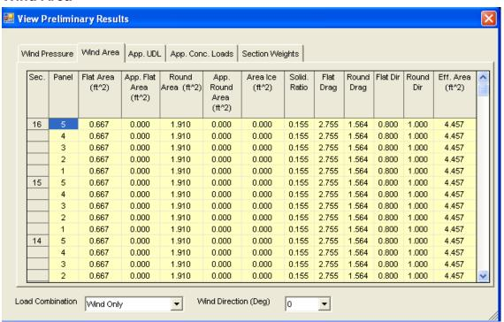
This screen shows flat and round areas of the structure and that of the appurtenances included as part of the structure in the calculations. Solidity ratios are also show for each panel and the calculated force coefficients (drag coefficients) for both flat and round members. Also the directionality factors and the total effective wind areas are shown for each of the load combinations and wind directions.
