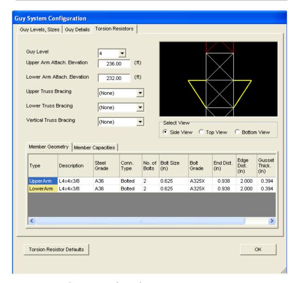
Torsion Resistor Geometry and members:
