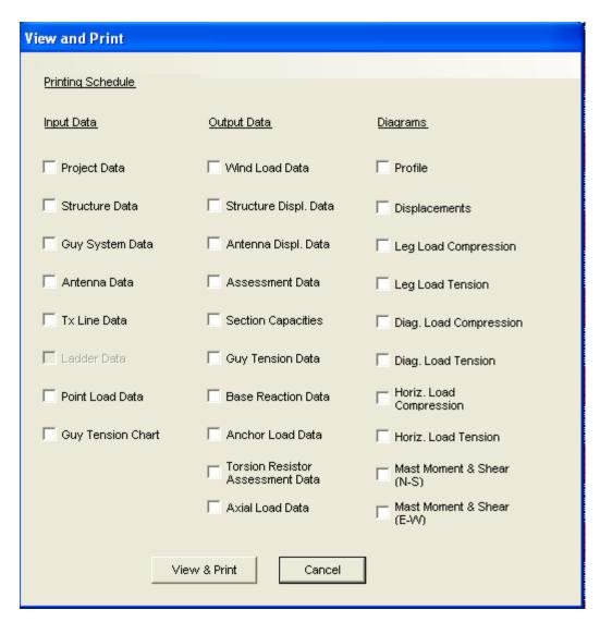
Note that for analysis including several load combinations and different wind directions as well the user has the option to select the required sections for printing and also the desired wind directions. This may result in a relatively large number of pages in the printout. By choosing the profile, the program prints a simple profile on which the project data, design specification, base reactions and tower geometry are printed in a graphical format.
