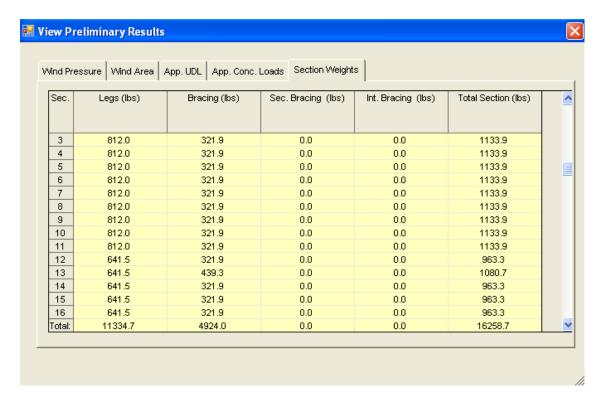
The section weights with divisions for Legs, Bracing, Secondary Bracing, Internal Bracing and Totals are shown in this grid.
