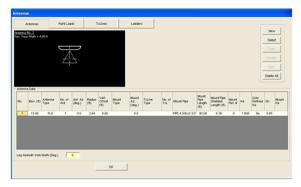
In this window the tower elevation is shown along with the plan cross-section at the marked antenna. To add a new antenna select **New** and a blank line with an antenna type (none) is shown. The user inputs the following data as defined below:
