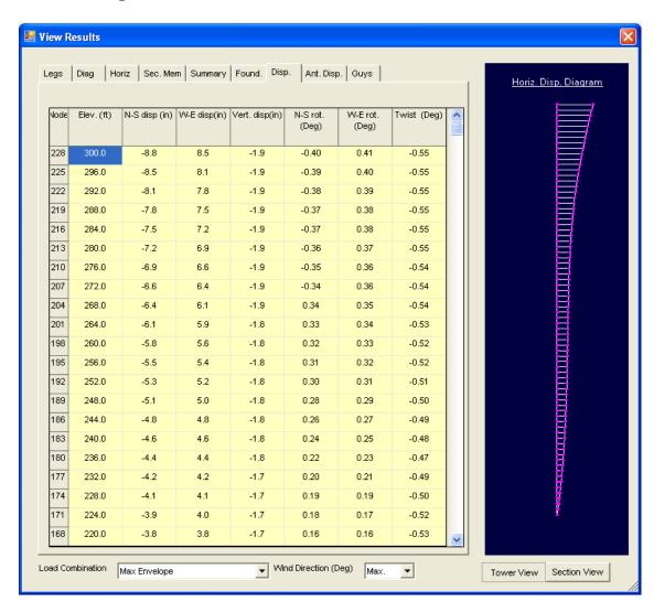
The displacements can also be viewed for the maximum envelope or any of the load combinations or wind directions.
