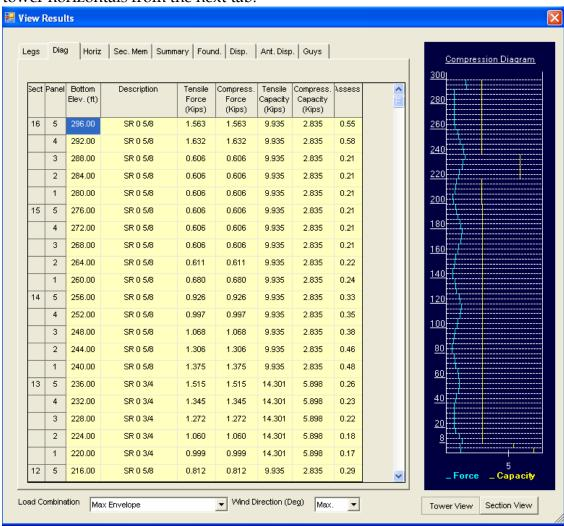
Also, on the bottom of the screen, the user may select the load combination for which results are to be displayed. Load combinations selected from the analysis menu are shown in the load combination list. Specific wind direction may be chosen or simply the envelope of the maximum values.
