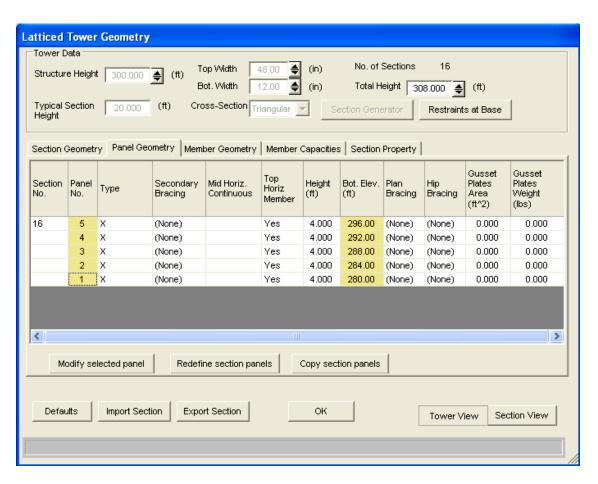
On the next Tab "Panel Geometry" the user can define the number, type, height of panels for the selected section. From the section column, other sections can be selected for Panel definition. Also on the same window the user can modify selected panels, change heights for different panels, redefine section panels and or copy section panels to other section(s).
