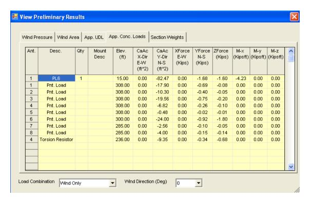
The appurtenances calculated concentrated loads are shown on this screen. The window shows the calculated flat and round areas in the direction of each axis and the corresponding forces and moments in the three axes. This value can be selected for each of the load combinations and wind directions.
