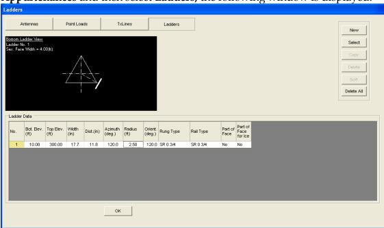
In this window the pole elevation is shown along with the plan cross-section at the bottom of the ladder. To add a new ladder select **New** and a blank line with a rail type, and rung type (none) is shown. The user inputs the following data as defined below:
