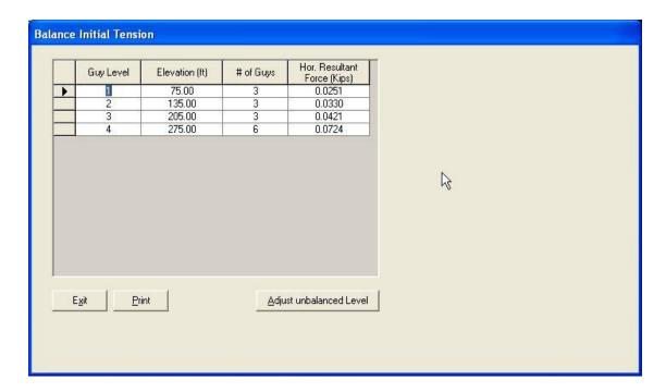
In case the horizontal resultants are considered too large (need for balancing) please click on "Adjust unbalanced Level" button for a selected guy level.
